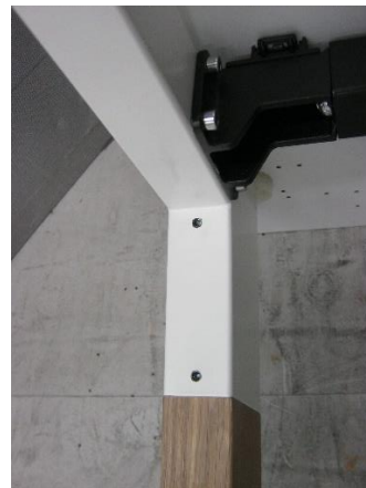
Photo 4: Tested sample 220609-4 of Techo Fount wood/steel leg - detail connection legs to frame
