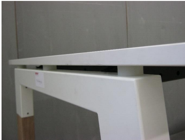
Photo 5: Tested sample 220609-4 of Techo Fount wood/steel leg - detail table top to legs side view
