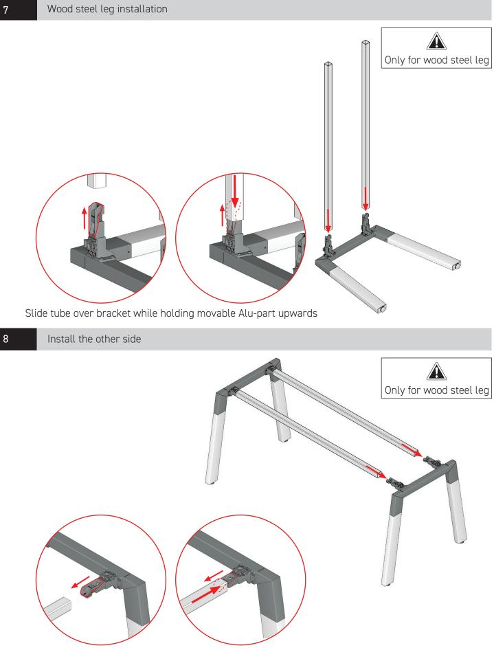
Push both tubes on both brackets simultaneously
